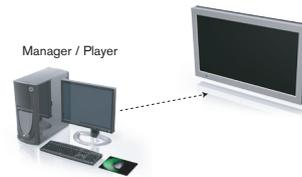
In this setup a separate computer is used for the playback. Playback is not interrupted by editing, and the manager computer can be used for other tasks.
